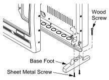
Figure 13 - Installing Base Feet
